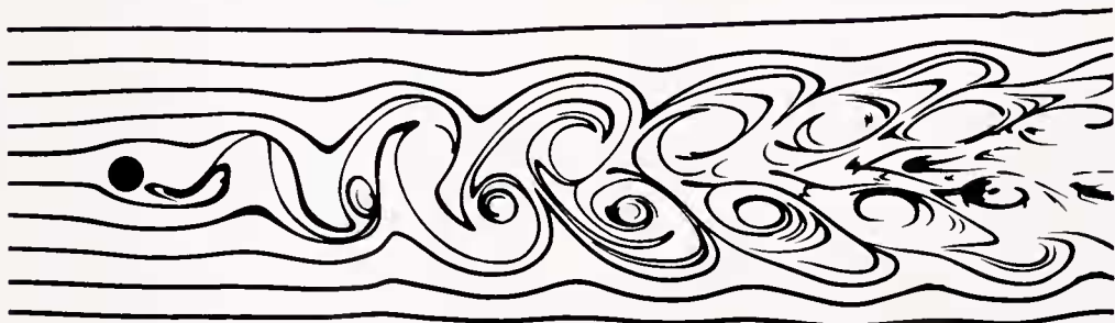
Figure 5. Artist's interpretation of a von Kármán vortex street in the wake of a circular cylinder, from a photograph by Peter Bradshaw (Van Dyke, 1982). Reynolds number ( Re ) of about 300 (where Re = LU/\nu ; L = characteristic length scale, U = characteristic velocity scale and \nu = kinematic viscosity of the fluid) is at the upper limit for stability of the vortex street, as indicated by the breaking up of the vortices at the downstream edge of the drawing. At lower Re a pair of vortices forms in the lee of the cylinder but is not shed into the flow, and at higher Re the vortices break up completely into a disorganized turbulent wake.
